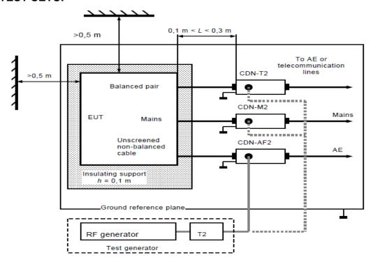
**Note:** 1. The CDNs and / or EM clamp used for real test depends on ports and cables configuration of EUT. 2. The EUT clearance from any metallic obstacles shall be at least 0.5m
